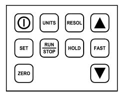
Press for power-on, press/hold for power off.
